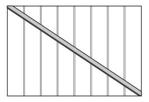
What is the length of a diagonal brace that could be used for a wall 9 feet high and 12 feet long?
