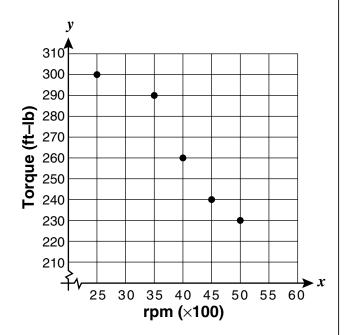
49 An engine is tested for torque output at different revolutions per minute.
